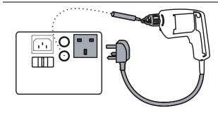
Figure 5. Insulation Test Connections
