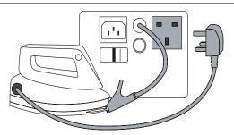
**Figure 4. Bond Test Connections**
