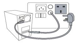
**Figure 7. Touch Current Connections**
