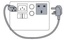
Figure 9. IEC-Lead Test Connections
